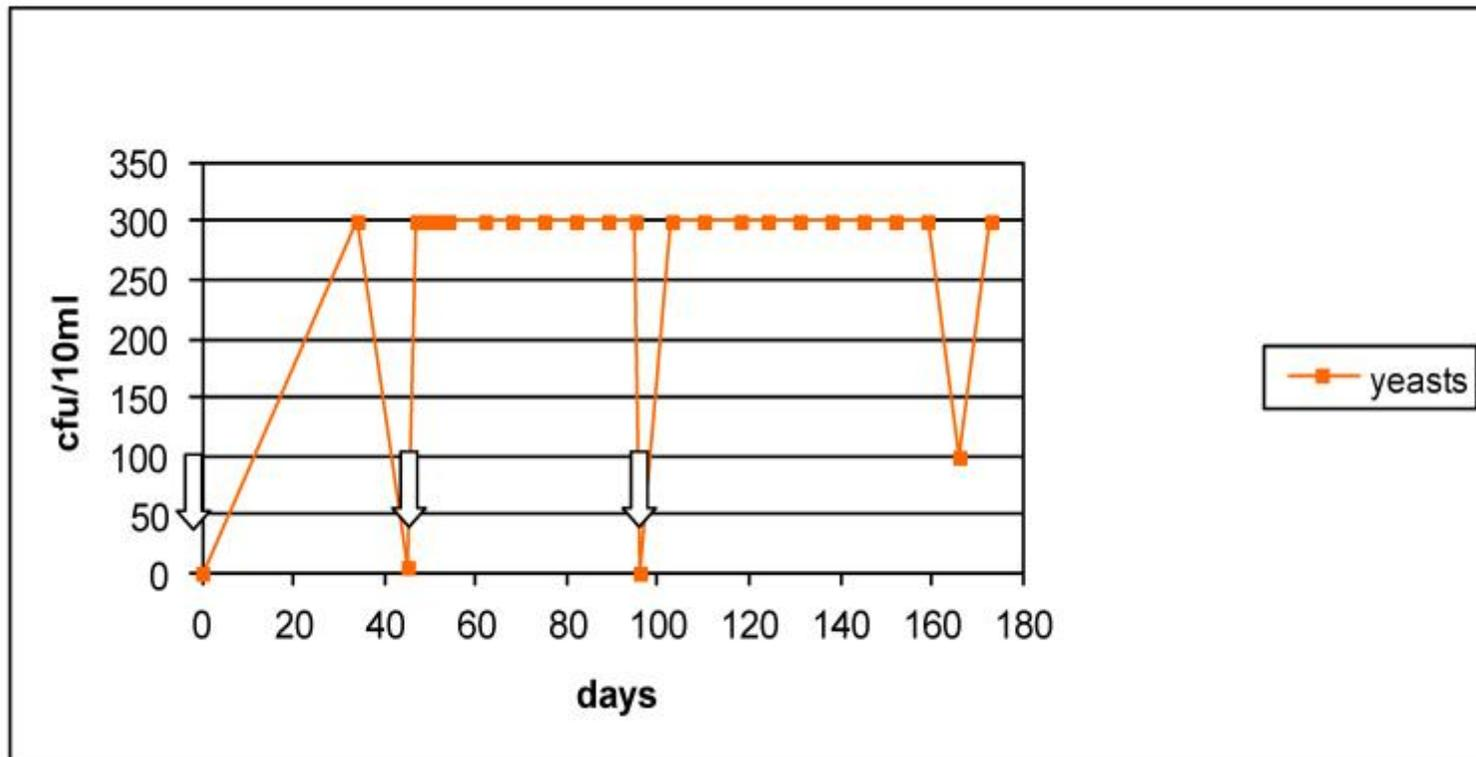
In the turbines of the older design with intensive biofilm formation, the PotoClean® technology was not effective
