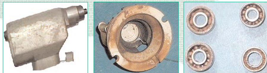
Fig. 3 to 5: Surface discoloration due to unsuitable detergents or water quality
