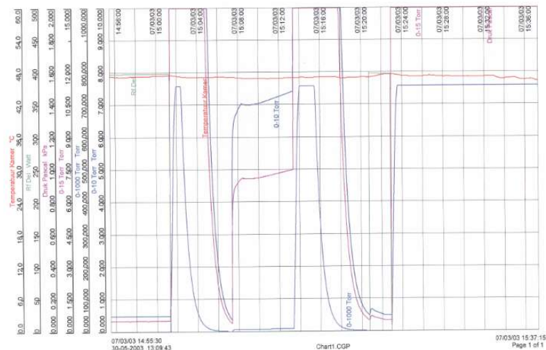
Fig. 6: a graphical display of a half cycle process during PQ of a STERRAD® 100S. (Red: Temperature; Green: RF energy delivered; Blue 1: pressure (measured by baratron 1: 0 – 1000 Torr or 0 – 133,41 kPa); Blue 2: pressure (measured by baratron 2: 0 – 15 Torr or 0 - 2 kPa) Time: every vertical bar represents 4 minutes).
