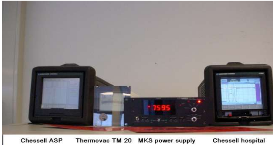
Fig. 3: instruments in parallel for monitoring low pressures and delivered RF energy during Qualification procedures
