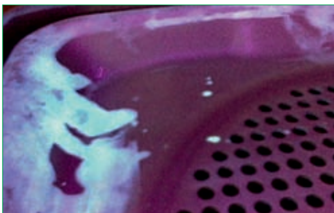
Photo 1 and 2: Visualisation of the wetted and unwetted surfaces using UV light
