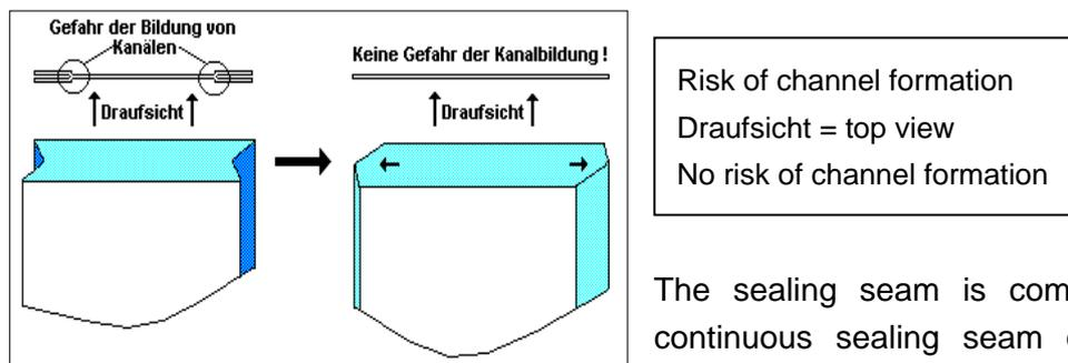
The sealing seam is composed of either a continuous sealing seam or of 3 to 4 fine grooves (whereby the sum of the area of the grooves must also be at least 8 mm). Individual grooves are easier to peel and are more noticeable (colour difference).
